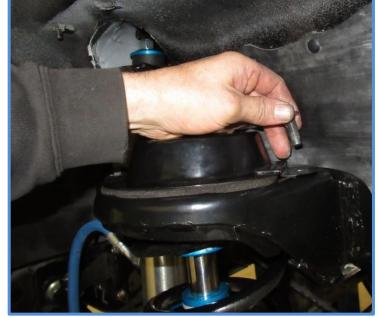
6. Install reservoir bracket. First place the reservoir in the clamp as shown. Then place the spacers in position over the holes for the coil bucket cap where you previously removed the bolts. Then place the reservoir bracket over the spacers and install the supplied M10 X 80mm bolts (CB3731) as shown.
