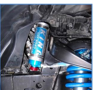
7. Now with the reservoir in place you can tighten the hardware starting with the three upper bolts using a 9/16 socket/wrench and then tighten the lower bolt using a 21mm socket.
