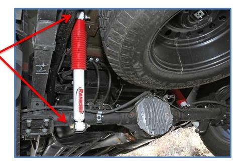
**NOTE:** When installing the new shocks, make sure that you have a driver and passenger side shock. This will insure that the off-set spacers are located in the right direction in order to space the shock away from the frame. Driver-side reservoir should face towards the rear and the passenger-side reservoir should face the front.
