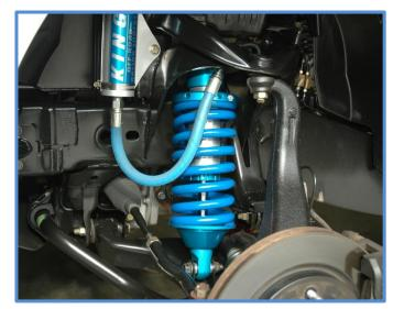
6. Once the shock is in and secure, slide the reservoir into the reservoir bracket and secure it with both hose clamps. (make sure the reservoir is centered in the bracket)
