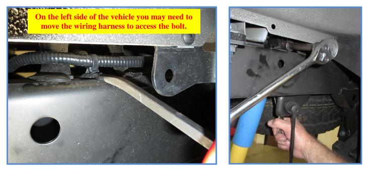
3. Install King Shocks by placing the end cap in the upper mount with the reservoirs facing away from the axle and the longer bearing spacer facing the frame. Install the factory hardware and tighten to factory specs.
