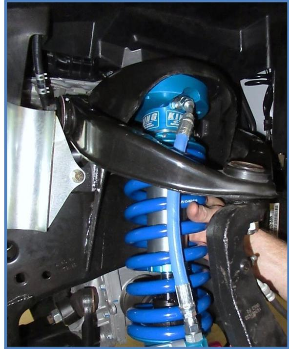
7. Install the provided 3/8 X 1" bolts (CB4701) with HD washers (CW1701) into the upper mount, thread the bolts in enough to hold shock in place but do not tighten yet. Install the factory bolt in the lower mount and tighten to factory specs, now tighten the upper mounting bolts to 35 ft/lbs.
