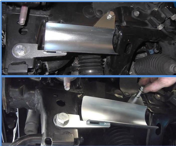
10. Install reservoir in the reservoir bracket with provided hose clamps as shown below.
