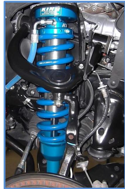
9. Install reservoir brackets using the provided hardware. Thread the 12mm bolt into the cross member, then insert the 7/16 x 3 3/4" bolt through the frame. Install washer, nut and tighten.
