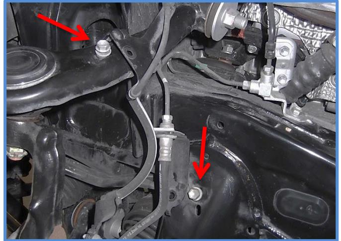
3. Keep a jack under the lower control arm on the side you are working on while disconnecting suspension components. Disconnect upper A-arms (A), tie rods (B), and lower shock mounting bolts (C).
