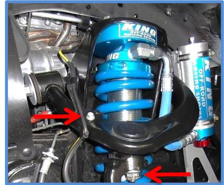
10. Install the sway bar to the threaded holes in the reservoir bracket using the 3/8" x 3/4" bolts and washers provided in the kit. The factory sway bar brackets are side specific and stamped "L" and "R" with an arrow that points toward the front of the vehicle. After the sway bar is mounted to the frame you can reconnect the sway bar links to the steering knuckle upright.
