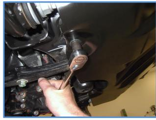
15. Now remove the sway bar mounting bolts at the frame using a 14mm socket. Do one side at a time.
