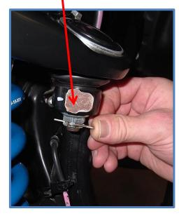
11. Reconnect tie rod end to the steering knuckle and tighten nut to factory specs. Be sure to insert the cotter pin through the castle nut and bend the ends as shown.
