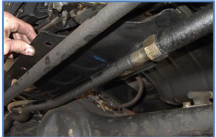
2. Remove the nuts on both ends of the factory steering stabilizer using a 17mm socket/wrench. You may need a ball joint tool or pickle fork to separate the tapered ends from the mounts.
