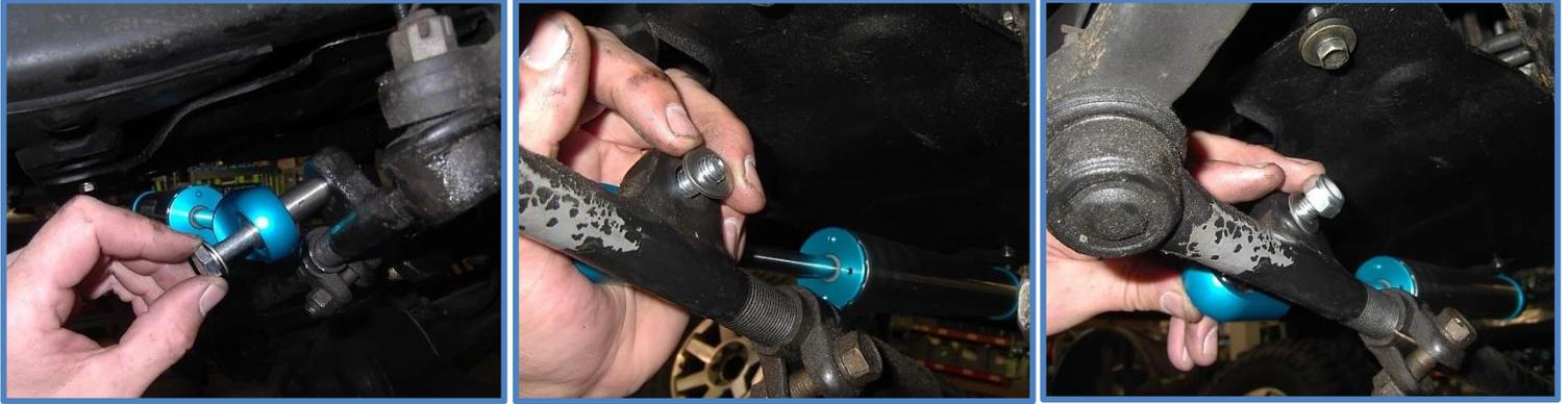
4. Install cylinder end to the factory mount on the opposite side. Insert the tapered spacer into the factory mount. Install the provided 10mm hardware as shown and tighten nut to 50 ft/lbs.
