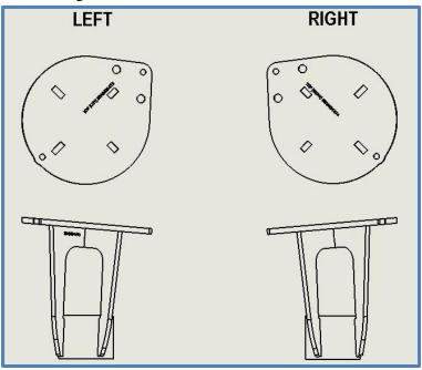
3. Install bump stop brackets using the provided 1/4 x 1" flat head screws, washers and nuts.
