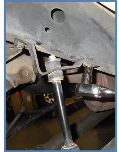
3. Place brackets in position on the frame lined up with the sway bar mounting holes. Brackets are side specific, be sure to mount brackets on the proper side (see photos below - Photos show right side being installed). Use the OE bolts you just removed to bolt the sway bar bracket back in place over the reservoir bracket.
