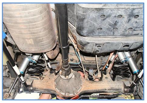
Remote reservoir applications require welding the reservoir mounts. Do Not Weld on vehicle with shocks installed. All welding must be performed by a certified welder. Reservoir location is up to the customer, be sure to check any clearance issues with hoses/reservoirs and moving suspension components before final install.
