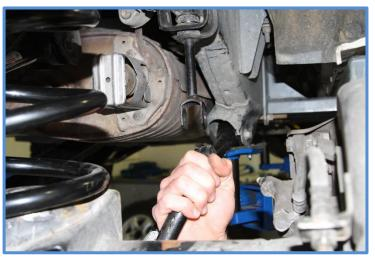
3. Install King Shocks - Remove the nut, washer, blue retaining washer and upper bushing. Insert the pin into the upper mount making sure the taller bushing is on the bottom next to the cylinder as shown below. Make sure the reservoirs are facing inward, towards the center of the vehicle.
