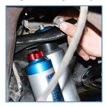
Important Note: The rubber bushings on your King shocks are different from each other. Make sure the taller bushing is on the bottom next to the body of the shock as shown. The silver washer between the rubber bushings represents the material thickness of the upper shock mount. It's important to tighten the nut only until the rubber bushings start to compress. There should be approximately 1/8" of the mounting pin protruding above the nut.
