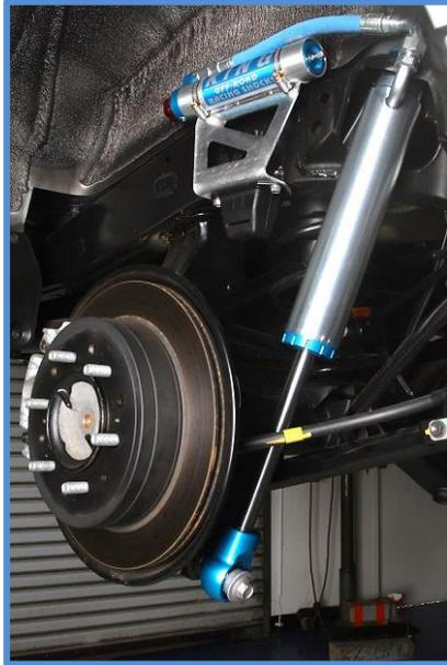
**Important Note:** The rubber bushings on your King shocks are different from each other. Make sure the taller bushing is on the bottom next to the body of the shock as shown. The silver washer between the rubber bushings represents the material thickness of the upper shock mount. It's important to tighten the nut only until the rubber bushings start to compress. There should be approximately 1/8" of the mounting pin protruding above the nut.
