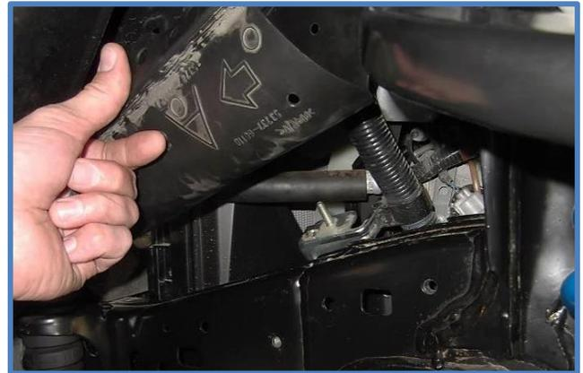
15. Bolt reservoir bracket to frame using the factory bolts and plastic piece as shown below.
