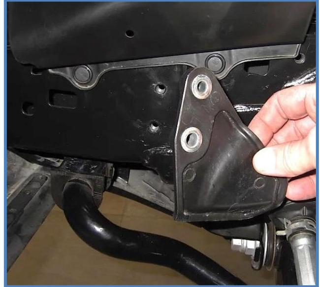
14. Pull the two plastic push pins from the plastic guard and flip up to install reservoir bracket and reservoir.
