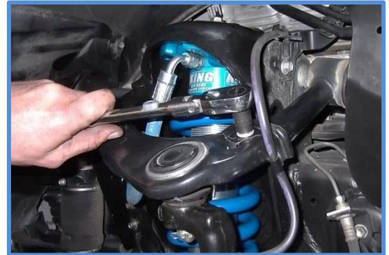
Reconnect the wiring harness bracket at the top of the coil bucket.
