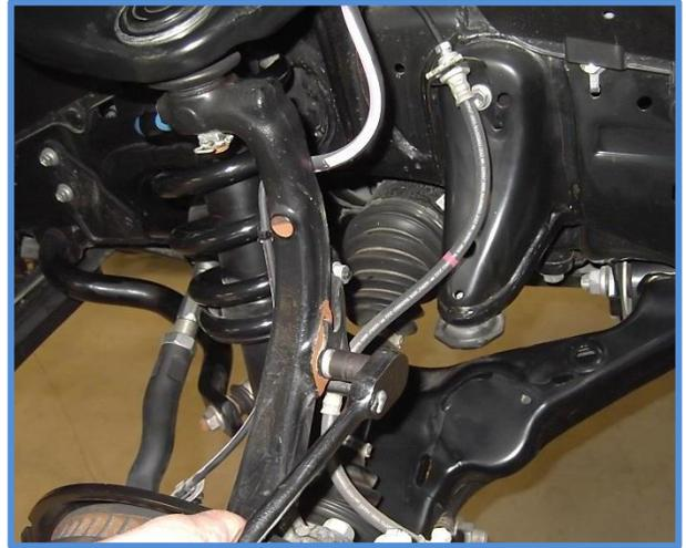
4. Pull the pin out of the ball joint stud in the upper control arm using needle nose pliers.
