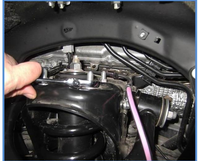
8. Remove the lower mounting bolt using a 22mm wrench and socket. Remove shock from vehicle.
