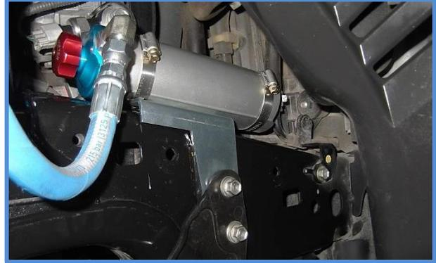
For KDSS Models... You may need to loosen the bracket that supports the hydraulic lines for the KDSS System on the left side of the vehicle. Remove bolt, install reservoir, then reinstall bolt and reposition bracket if necessary and tighten everything once positioned properly.
