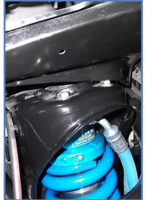
10. Install the factory lower mounting bolt and check clearance at full droop as shown in step 11 on the next page. Make any necessary adjustments, then install factory hardware and tighten to factory specs.
