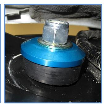
7. Place the rod end on the lower mounting stud and install the factory bolt. Torque bolts to factory specs
