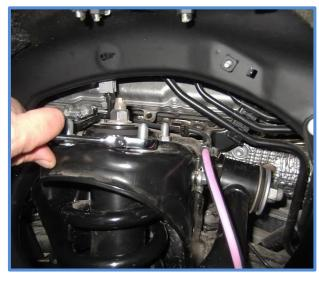
8. Remove the lower mounting bolt using a 22mm wrench and socket. Remove factory shock.
