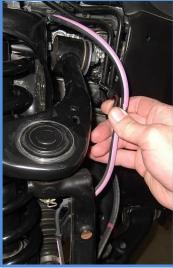
4. Unbolt the ABS/brake line bracket on the spindle and frame using a 12mm wrench/socket.
