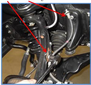
5. Pull the pin out of the ball joint stud in the upper control arm using needle nose pliers.
