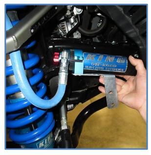
16. Bolt reservoir bracket to frame using the factory bolts and plastic piece as shown below. Once the bracket is secure, adjust reservoir as needed and tighten clamps using the 1/4 x 1" SHCS (CB1501).
