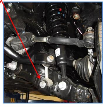
2. Disconnect the tie rod end by first removing pin using needle nose pliers, then remove nut using a 24mm socket and separate tie rod from steering knuckle.
