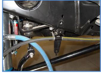
10. Slide reservoir into reservoir bracket. Install the 1/4 x 1" socket head cap screws, leave loose for now you will have to adjust the hose and tighten clamps last.
