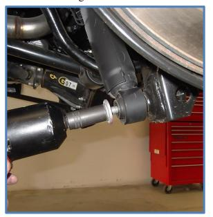
2. Remove upper nut using a 22mm wrench. You may need to hold the top of shock with large pliers.
