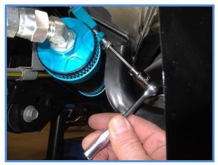
11. Place loop clamp on hose as shown and use the provided 8mm x 25mm flanged head bolt to mount the loop clamp and the parking brake cable holder to the frame.
