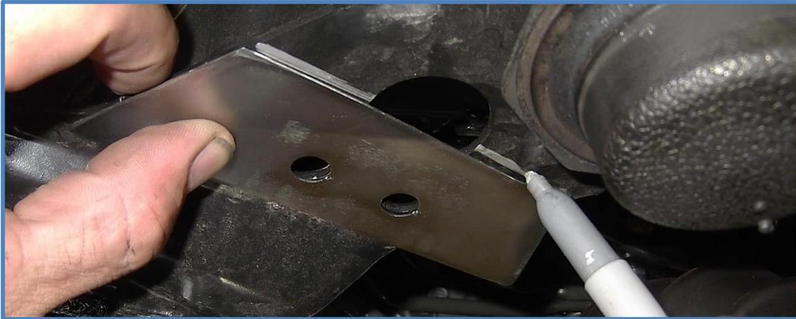
4. Now connect the top and bottom lines on the side of the bracket as shown.
