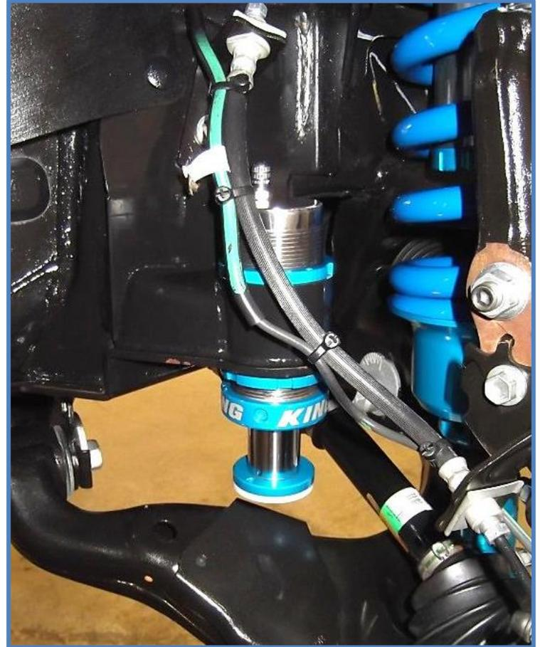
**DOUBLE CHECK ALL HARDWARE:** Reinstall shocks and any other components that were removed or disconnected during bump stop install. Make sure everything is installed correctly and all hardware is tight before reinstalling tires. Install tires, remove jack stands and lower vehicle to the ground. Recheck all hardware and lug nuts after 100 miles and periodically after that as part of routine maintenance.
