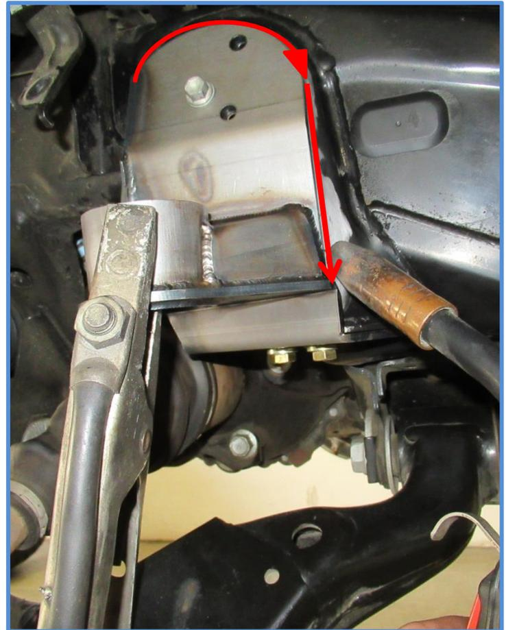
11. When welding is complete, prep and paint all bare metal to protect from rusting.
