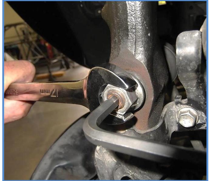
4. Pull the pin from the upper ball joint, loosen nut using a 19mm Socket and separate upper control arm from the steering knuckle.
