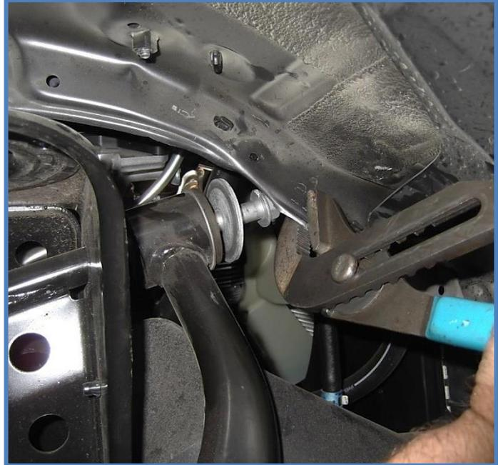
**Be careful not to damage the wiring harness and AC lines on the inside of the fenders when removing the bolt.**
