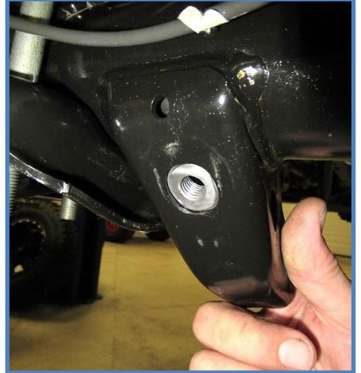
3. Place the shock mount extension over the existing mount and line up the holes in the bracket with the holes on the existing mount. Thread the 1/2 X 1" bolt (CB4704) with washer (CW1702) into the square nut and leave loose for now.
