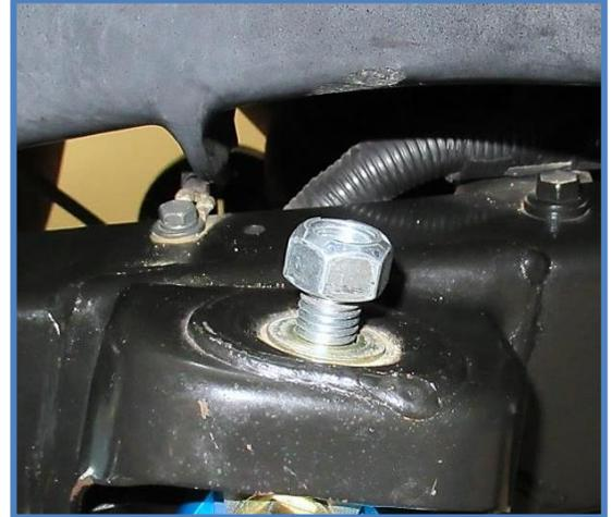
7. Place the rod end in the lower mount and install the 1/2 X 2-3/4" bolt (CB4730) with washer (CW1702). Be aware that these shocks have offset bearing spacers, the longer spacers should be towards the frame which offsets the shock out towards the wheel, this is to provide clearance between the shock and the leaf spring. Make sure the longer spacers are towards the frame. Install the washer (CW1702) and thin nylock nut (CN2800) and tighten both shock mount bolts to 90 ft-lbs.
