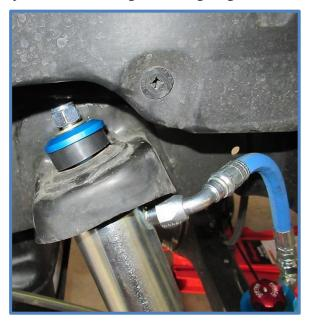
7. Place the rod end into the lower mount. Install the factory bolt and nut finger tight.
