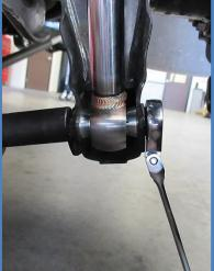
Important Note: The rubber bushings on your King Shocks are different from each other. Make sure the taller bushing is on the bottom next to the body of the shock as shown. The silver washer between the rubber bushings represents the material thickness of the upper shock mount. It's important to tighten the nut only until the rubber bushings start to compress. There should be approximately 1/8" – 3/16" of the mounting pin protruding above the nut.
