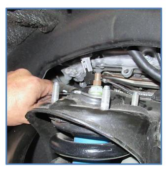
7. Install King Shocks. (Shocks are side specific) First place the shock into the upper mount and insert upper mounting studs into upper mount on vehicle. Photos below show the left side.
