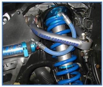
8. Place the rod end into the mount on the lower control arm, you may need help pushing down on lower arm while inserting rod end. Make sure the longer bearing spacer is facing forward.
