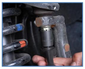
4. Remove lower shock mounting bolt using a 22mm wrench and socket.
