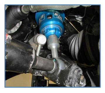
11. Connect upper control arm to the spindle following the instructions that came with your control arms. Then reconnect ABS and brake line brackets. The Total Chaos arms shown here provide a tab and hardware to mount the factory ABS line bracket to the new control arm.
