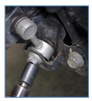
NOTE: To make sure sway bar does not make contact with the shocks, we recommend rounding off the corners of the sway bar as shown in the photo. Trim, grind and paint the sway bar ends while the shocks are removed.
