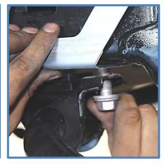
13. Slide two of the reservoir clamps onto the reservoir (see photo's for proper orientation). Position the reservoir over the reservoir bracket and install the 1/4 X 1/2" BHCS (CB2420). Use a 5/32 allen wrench to secure clamp to bracket. Then install the 1/4 X 1" SHCS (CB1501) to tighten clamp, center reservoir and adjust as needed. Tighten clamp using a 3/16 allen wrench. See step 16 for note on trimming plastic on right side.
