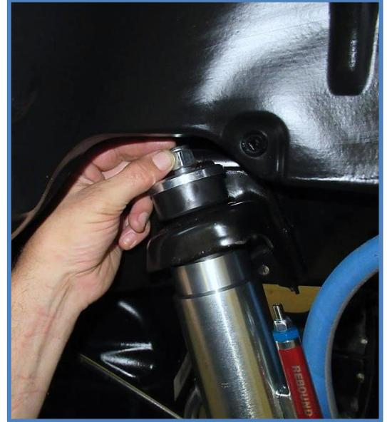
8. Tighten the upper nut using a 15/16 wrench. You should tighten the nut until the bushings start to compress, there should be about 1/8 – 1/4" of thread protruding past the nut. Do Not Overtighten!
