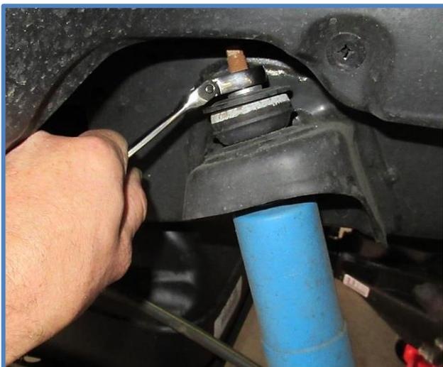
2. Next remove the lower nut and bolt using a 17mm wrench and socket and remove shocks.
