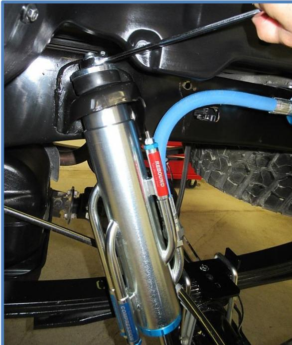
9. Place the rod end in the lower mount and reuse the factory nut and bolt. Tighten nut to factory specs. (66 ft-lbs.) using a 17mm wrench and socket.
