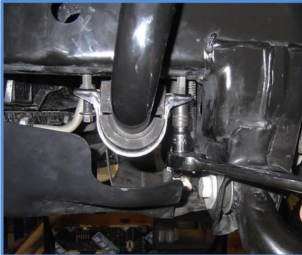
13. Using the factory bolts, attach the sway bar plates to the frame with the threaded holes towards the front of the truck as shown below.
