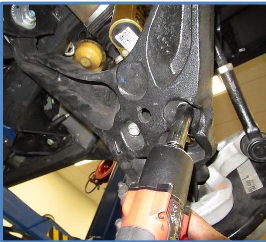
5. The shock is now hanging from the upper mount, be sure to hold on to it as you remove the three nuts from the upper mount using an 18mm wrench or socket.
