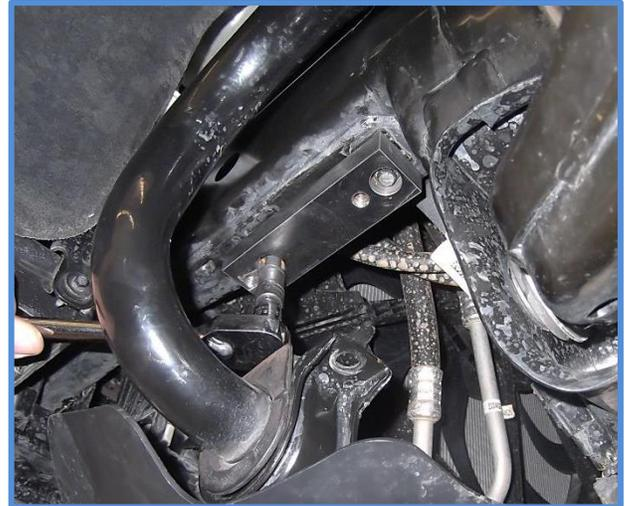
14. Bolt the sway bar to the sway bar plate using the supplied 3/8" x 3/4" bolts and tighten with a 9/16 socket.
