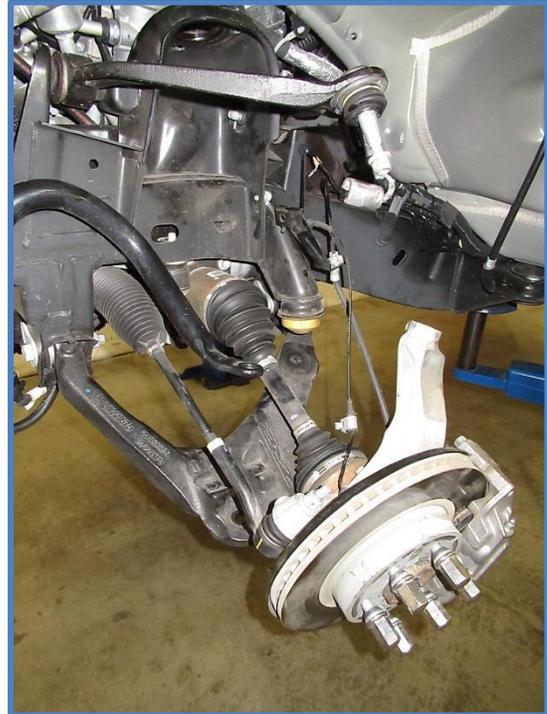
7. Installing King Shocks – Be aware the shocks are side specific, make sure you are installing the proper shock on the correct side (see pics below for reference). Place the shock in position on the vehicle and install the provided 10mm lower mounting bolts w/washers. Insert bolts up through the lower mount, install the washers and nuts and tighten to 40 ftlbs.
