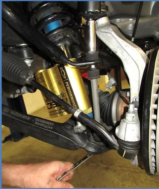
3. Remove the nut from the upper control arm ball joint using an 18mm socket and separate the upper control arm from the knuckle/spindle.
