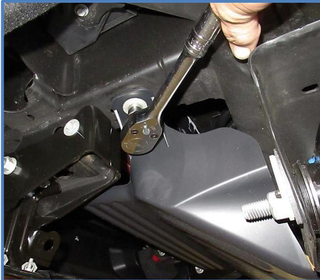
15. Remove the clip in the frame that the bolt was attached to. The reservoir bracket will mount to frame using this hole.
