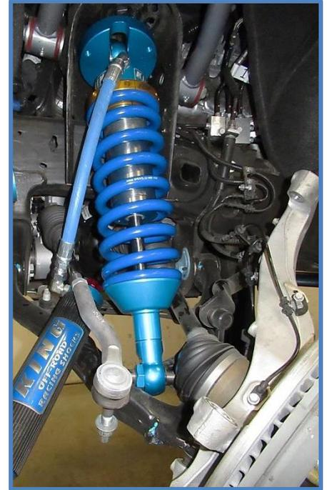
9. Install the provided 3/8 x 1" bolts (CB4701) with HD washers (CW1701) in the upper mount and tighten to 35 ft. lbs.
