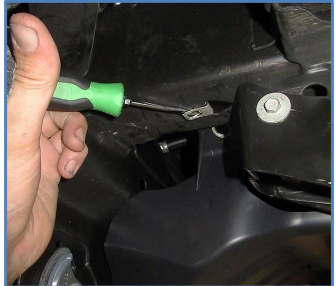
16. Attach reservoir clamps to the reservoir brackets using the provided 1/4 X 3/4" FHCS (CB5520). Attach clamps as shown below and tighten screws using a 5/32 Allen wrench.
