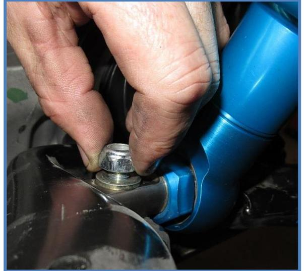
11. Reconnect upper control arm to knuckle and tighten hardware to factory specs. Connect aftermarket upper arms using the instructions provided with your control arms.
