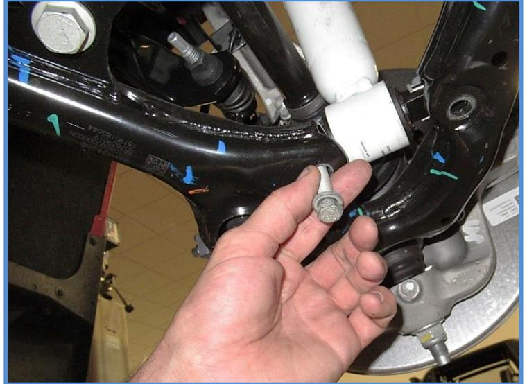
3. Remove the upper mounting nuts using an 18mm wrench or socket. You will have to move the plastic wiring harness housing out of the way to access the upper nuts.
