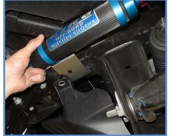
18. Using the factory bolt you just removed and the 90° nut plate provided in the kit, secure the reservoir bracket to the frame. The reservoir bracket will sit against the frame and the plastic piece will go over the reservoir bracket as shown. Install the factory bolt and tighten.
