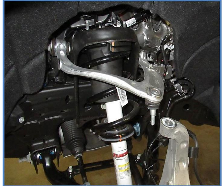
5. Remove nut from tie rod end using a 21mm wrench or socket and separate tie rod end from knuckle.
