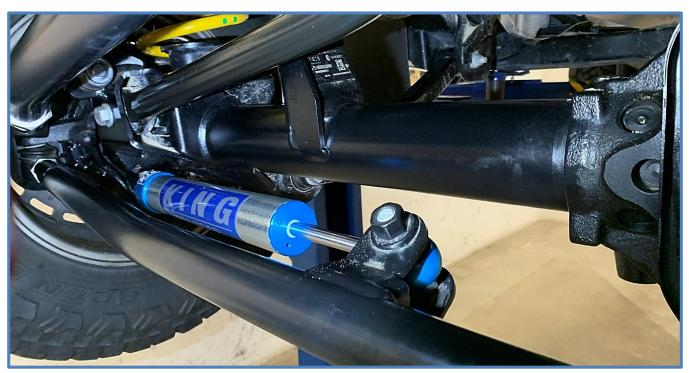
Double check your install, make sure the stabilizer is mounted properly and all hardware is tight. Recheck the hardware after 50 miles and periodically after that as part of routine maintenance
