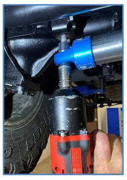
5. Place the rod end into the mount on the tie rod. Install the factory bolt and torque to factory specs.
