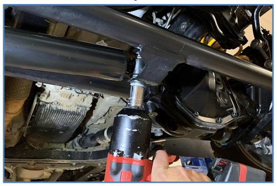
3. Install King stabilizer as shown. Place the cylinder end of the stabilizer on the axle mount with the longer bearing spacer facing the mount.
