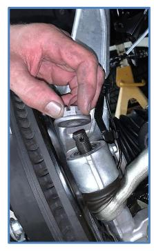
4. Remove lower shock mounting bolt using a 22mm wrench and socket.
