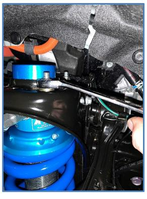
8. Insert the factory lower mounting bolt through the lower mount. Install the washer and nut, then tighten to factory specs.
