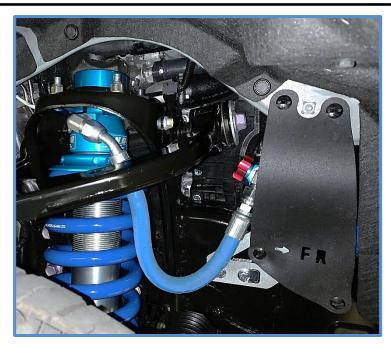
21. Install tires and lower vehicle to the ground, then install sway bar link to the lower mounting stud. Install the factory bolt and torque bolts to factory specs using a 19mm socket.
