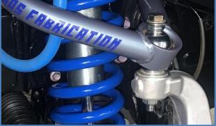
11. Reconnect the brake and ABS lines to the <u>frame</u>, <u>upper control arm</u> and <u>knuckle</u>. Tighten bolts to factory specs using a 12mm socket.
