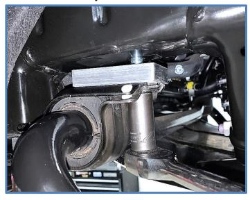
19. <u>Install Skid Plate Spacers</u> – First remove the two bolts in the front of skid plate using a 12mm socket.
