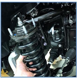
6. <u>Install King Shocks</u> – Be aware shocks are side specific. Hose and reservoir will go towards front of vehicle. See final install pictures for proper orientation. Place shock in position on the vehicle by first maneuvering top of shock into upper mount. Then pry down on lower control arm and place rod end in the lower mount.
