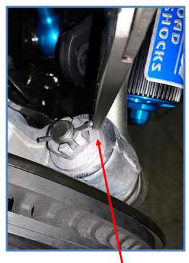
10. Connect upper control arm after connecting tie rod. Tighten nuts to factory specs. Reinstall the Pins.
