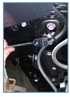
2. Remove pin from upper ball joint, loosen nut with a 19mm socket. Separate upper A-arm from spindle.
