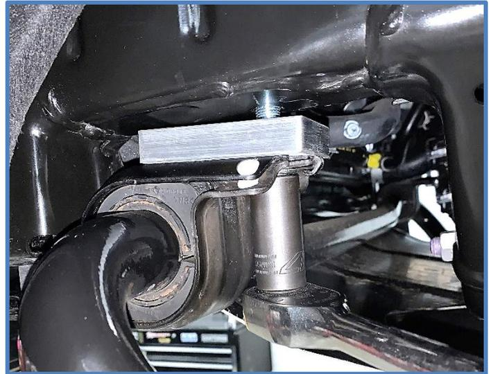
19. **Install Skid Plate Spacers** – First remove the two bolts in the front of skid plate using a 12mm socket.
