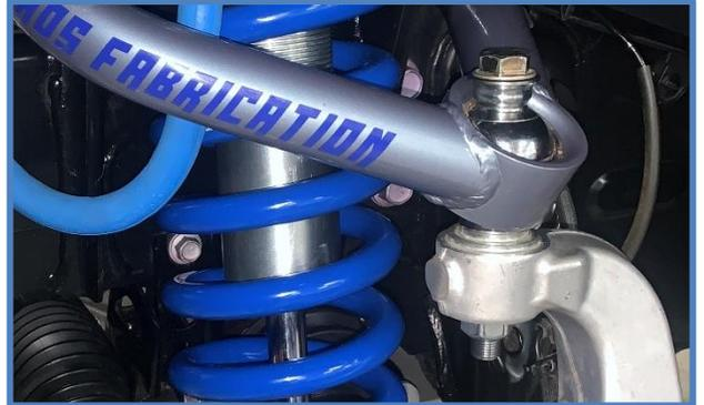
11. Reconnect the brake and ABS lines to the frame, upper control arm and knuckle. Tighten bolts to factory specs using a 12mm socket.
