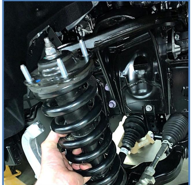
6. **Install King Shocks** – Be aware shocks are side specific. Hose and reservoir will go towards front of vehicle. See final install pictures for proper orientation. Place shock in position on the vehicle by first maneuvering top of shock into upper mount. Then pry down on lower control arm and place rod end in the lower mount.
