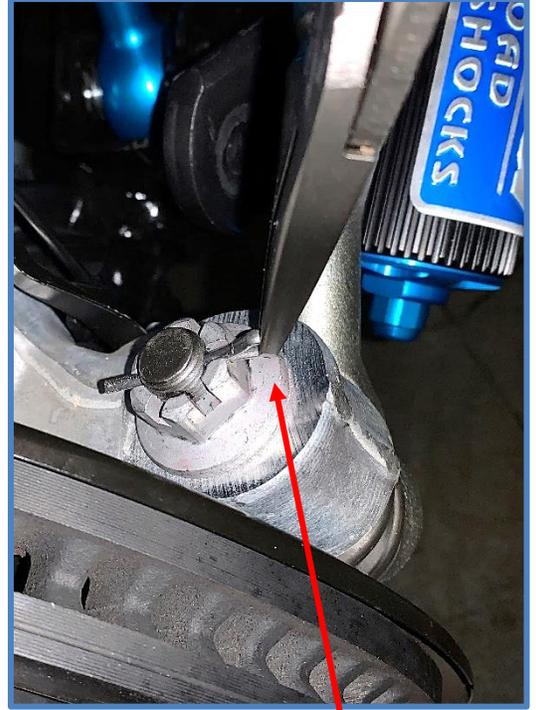
10. Connect upper control arm after connecting tie rod. Tighten nuts to factory specs. Reinstall the Pins.
