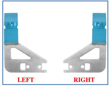
9. Insert the Backing Plate (25049-040) into the rectangular hole in frame with the rounded corners facing towards the front of vehicle. Flip the plate out with thumb as shown below and slide forward to hold in place.
