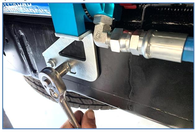
13. Install the 1/4 x 1" SHCS (CB1501) in the reservoir clamp. Adjust reservoir to its final position (See photos below) and tighten bolt using a 3/16 Hex Key. (For shocks with Compression Adjusters check clearance here.)
