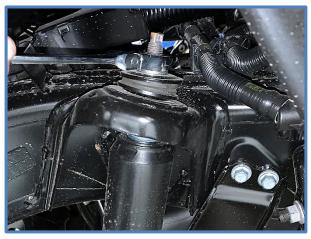
3. <u>Install Brake Line Bracket</u> – Remove the bolt holding the factory brake line bracket using a 12mm socket. Attach the provided Brake Line Bracket to the factory location using the factory bolt, then attach the factory brake lines bracket to the new bracket as shown below using the supplied 8mm bolt (CB3825) place the supplied washer and nut on the bolt and tighten.
