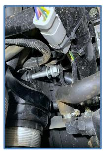
3. <u>Install King Shocks</u> - Place the shock in position on the vehicle; place rod end into the lower arm and maneuver the top of shock into the upper mount on the vehicle and install the factory upper bolt and nut.
