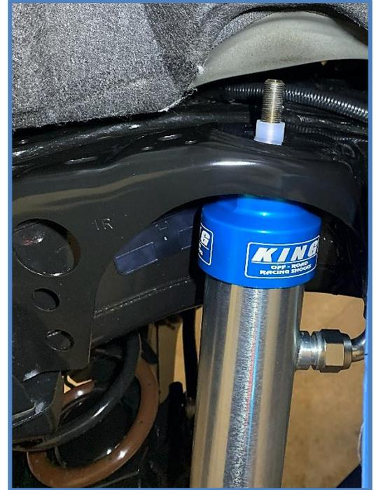
5. Place the upper bushing on the mounting stud followed by the blue retaining washer, 1/2" washer and nut. Apply anti-seize to the threads and thread the nut on finger tight for now to hold the shock in place.
