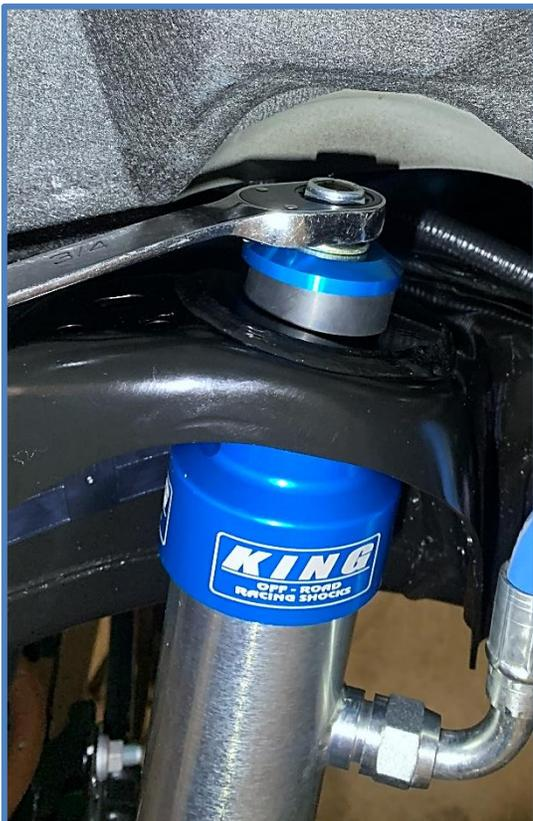
**Important Note:** The rubber bushings on your King shocks have raised center sections that should be facing each other when installed on vehicle. Taller bushing should be on bottom next to cylinder. The silver washer between the rubber bushings represents the material thickness of the upper shock mount. It's important to tighten the nut only until the rubber bushings start to compress. There should be approximately 1/8 – 3/16" of the mounting pin protruding above the nut.
