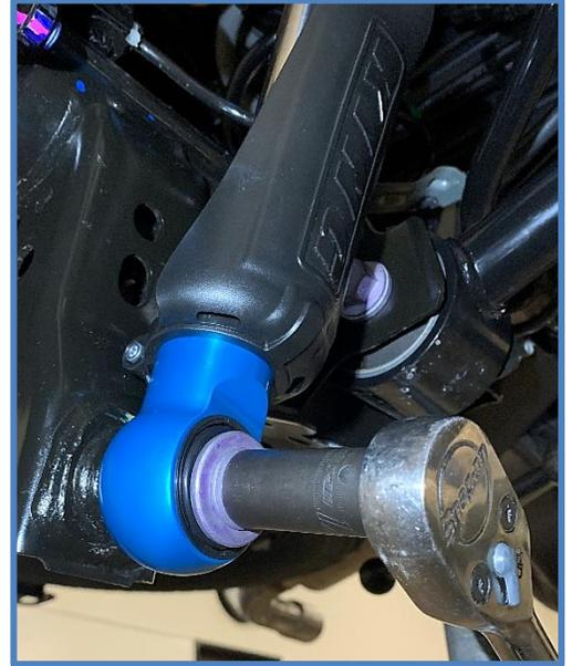
7. Tighten upper nut using a 3/4" wrench.
