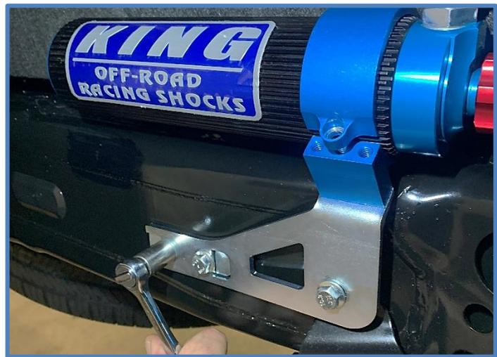
13. Install the 1/4 x 1" SHCS (CB1501). Adjust reservoir to its final position and tighten bolt using a 3/16 Hex Key.
