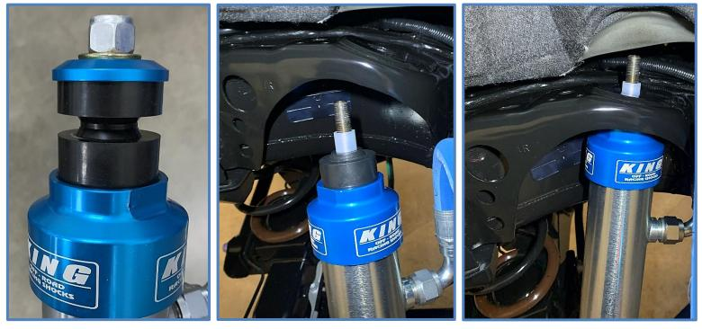
5. Place the upper bushing on the mounting stud followed by the blue retaining washer, 1/2" washer and nut. Apply anti-seize to the threads and thread the nut on finger tight for now to hold the shock in place.
