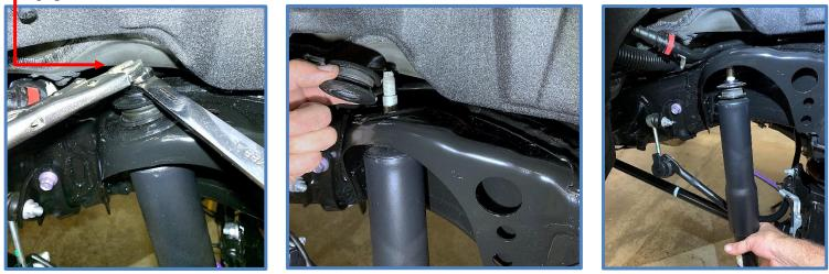
3. <u>Install Brake Line Bracket</u> – Remove the bolt holding the factory brake line bracket using a 12mm socket. Attach the provided Brake Line Bracket to the factory location using the factory bolt, then attach the factory brake line bracket to the new bracket as shown below using the supplied 8mm bolt (CB3825) place the supplied washer and nut on the bolt and tighten.
