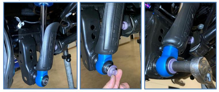
7. Tighten upper nut using a 3/4" wrench.
