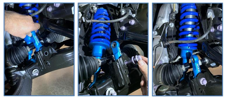
3. Use the supplied M16 bolt (CB3839) with washers (CW1803) and nuts (CN3003) to attach the sway bar link to the sway bar. Place one of the washers on the bolt followed by the short spacer and install through the sway bar link.
