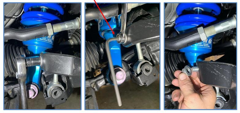
3. Remove factory sway bar links from both sides of vehicle.
