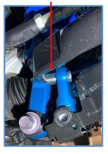
6. Install the provided 14mm X 80mm Bolt (CB3836) with washer (CW1805) through the sway bar link and into the sway bar so that the longer spacer is facing the sway bar and the nut will be on the outside of the sway bar. Install a washer and nut (CN3007) and thread nut on finger tight for now.
