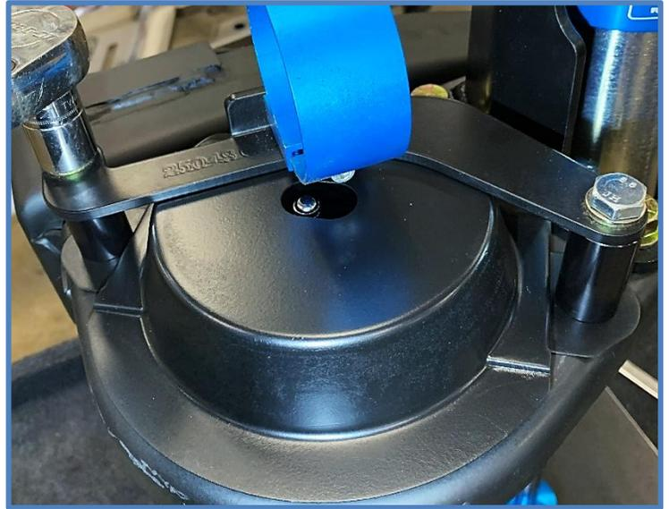
13. Slide reservoir into the reservoir clamp. Adjust the reservoir to the desired position and install the provided 1/4 X 1" SHCS (CB1501) in the reservoir clamp, tighten the clamp using a 3/16 allen wrench.
