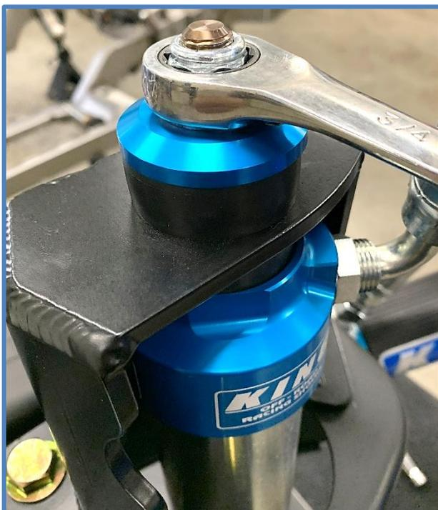
**Important Note:** The rubber bushings on your King shocks are different from each other. Make sure the thinner bushing is on the bottom next to the body of the shock as shown. The silver washer between the rubber bushings represents the material thickness of the upper shock mount. It's important to tighten the nut only until the rubber bushings start to compress. There should be approximately 1/8" of the mounting pin protruding above the nut.
