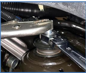
3. <u>Install Brake Line Bracket</u> – Remove the bolt holding the factory brake line bracket using a 12mm socket. Attach the provided Brake Line Bracket to the factory location using the factory bolt, then attach the factory brake line bracket to the new bracket as shown below using the supplied 8mm bolt (CB3825) place the supplied washer and nut on the bolt and tighten.
