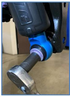
11. Tighten upper nut using a 3/4" wrench.
