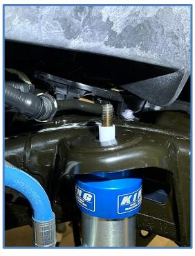
9. Place the upper bushing on the mounting stud followed by the blue retaining washer, 1/2" washer and nut. Apply anti-seize to the threads and thread the nut on finger tight for now to hold the shock in place.
