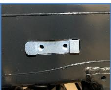
7. Place the reservoir bracket over the backing plate and thread two of the 8mm bolts (CB3825) into the backing plate and leave bolts loose for now, you will need to tilt the bracket out away from the frame to slide reservoir into clamp. Tighten these bolts after installing the reservoir.
