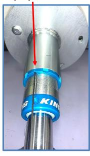
5. Place the King bump stop mount in the factory location and use the provided 10mm washer (CW1802) and 10mm nut (CN3004) to attach the bump stop mount. Tighten nuts using a 17mm wrench or socket.
