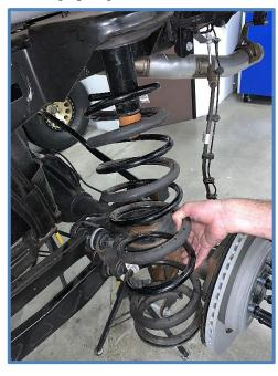
3. Remove the two nuts from the factory bump stop mounting studs using a 16mm wrench/socket and remove the factory bump stop mount. Remove the rubber spring isolators and make sure to install them on the same side as they were removed from when reinstalling springs.
