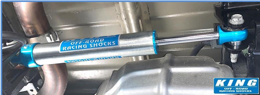
**DOUBLE CHECK ALL HARDWARE:** Make sure the shock is installed properly and all hardware is tight. Recheck all hardware after 100 miles and periodically after that as part of routine maintenance.
