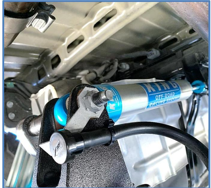
3. Place the shaft end in the mount on the crossmember, install the original bolt and tighten to factory specs.
