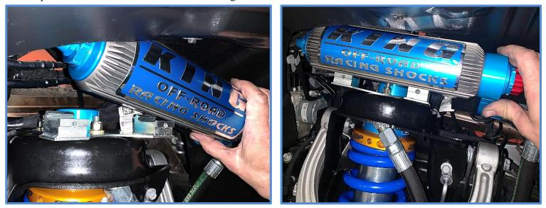
22. Install the retaining clips with the provided 1/4-20 X 1.75 SHCS (CB1508). Make sure the retaining clip engages in the groove on the reservoir, center the reservoir on the mount and tighten screws with a 3/16 Hex Key.
