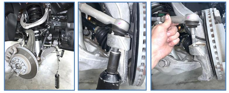
5. Separate upper control arm – Loosen nut using a 21mm wrench or socket, (you may need to hold the stud
