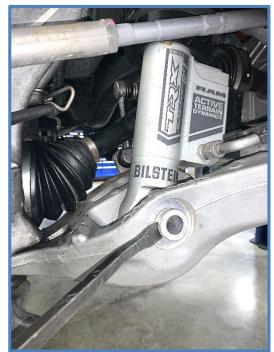
9. Disconnect upper control arm and remove shocks from vehicle.
