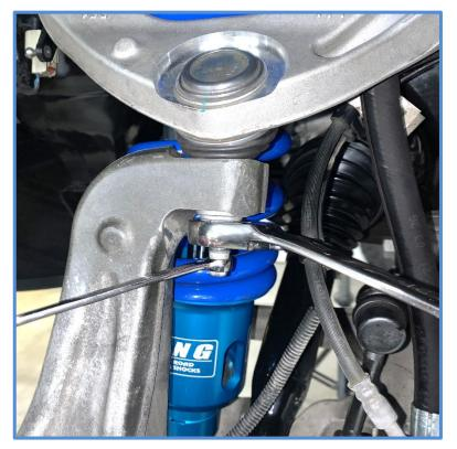
17. Attach the reservoir bracket to the upper mount. Place reservoir bracket over the upper mounting studs as shown below.
