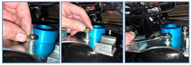
19. Tighten lower mounting bolt and torque to factory specs.
