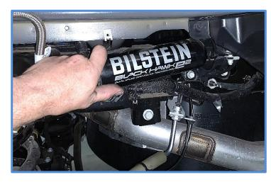
3. Unclip the hose from the studs on top of the upper coil mount.
