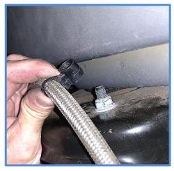
4. Remove the lower mounting bolt using a 21mm wrench and socket.
