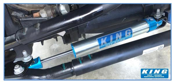
**DOUBLE CHECK ALL HARDWARE** - Make sure stabilizer is installed correctly and all hardware is tight.
