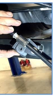
9. Finally attach parking brake cable to the new bracket on axle as shown below using the provided hardware.
