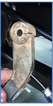
7. Next remove the cable from the holder on the left lower trailing arm. Pry the loop open enough to remove cable. Upper portion of bracket will not be reused, you can modify as shown in next step or leave as is...
