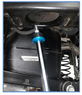
11. Place the cylinder end in the mount on the axle with the reservoirs facing forward. Install the factory bolt, tighten and torque to factory specs. Make sure there is room for the reservoir and brake cable on right side.
