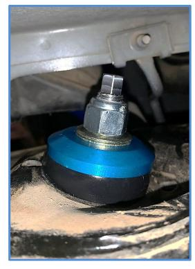
Important Note: The rubber bushings on your King shocks are different from each other, the bottom bushing has a raised center section that should be facing up when installed on vehicle. The silver washer between the rubber bushings represents the material thickness of the upper shock mount. It's important to tighten the nut only until the rubber bushings start to compress.
