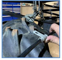
5. Attach the provided parking brake cable relocation bracket to the top of axle housing as shown below, reuse the factory bolt along with the bolt from the kit to attach bracket.
