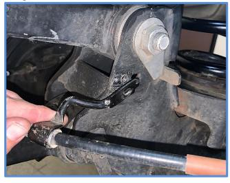
3. Pry open the loop on the parking brake cable holder and remove the cable holder from the cable. This piece will not be reused.
