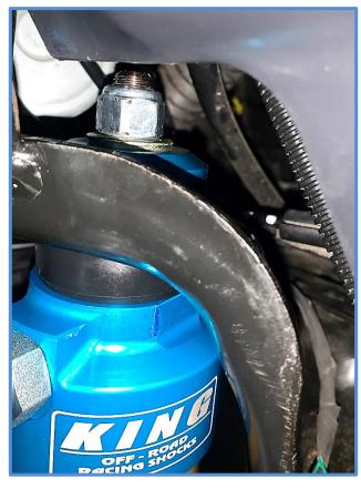
12. Tighten upper nut using a 3/4" wrench.
