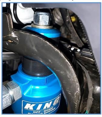
10. Use jack to position axle then place rod end in the lower mount, install the factory hardware and tighten to factory specs.
