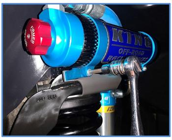
Your installation should look similar to the photo below. Make sure everything is installed properly and double check all hardware. Install tires, remove jack stands and lower vehicle. Recheck all hardware and lug nuts after 100 miles and periodically after that as part of routine maintenance.
