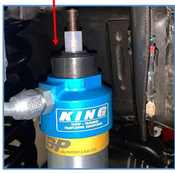
8. Slide reservoir into the reservoir clamps as shown below, then place shock into the upper mount.
