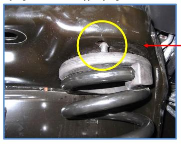
6. Place the reservoir brackets in position on the rubber isolators so the hole for the locating pin lines up.
