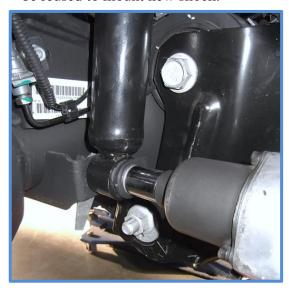
5. Lower the axle until you can slide the reservoir bracket between the rubber spring isolator and the upper spring mount.
