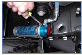
Some models have a plastic piece that needs to be trimmed slightly for the reservoir to fit.
