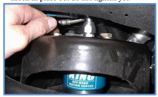
14. Line up the lower mount and use the supplied 12mm bolts and washers along with the factory nuts. Install hardware but do not tighten yet.
