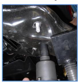
5. Using a 15mm socket, remove the three nuts from the top of the shock assembly and remove the shock.
