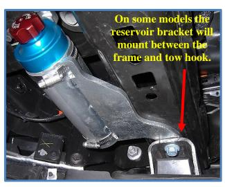
7. <u>2wd</u> – For 2wd models and vehicles without tow hooks, you may need to remove bumper to install reservoir brackets if access to mounting points are not available. First remove the two bolts for the lower air dam using a 13mm socket and remove the air dam.
