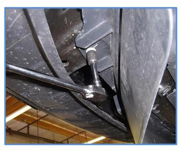
8. Open the hood to access the hood latch bolt and two other bolts that need to be removed. Use a 10mm socket for the hood latch bolt and an 8mm socket for the other two bolts. Also, make sure the hood latch cable is unclipped from the fascia.
