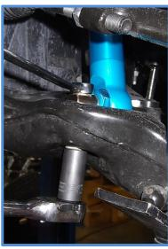
17. Reconnect the upper A-arm and torque to factory specs.
