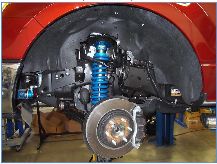
Alignment is critical: A professional alignment must be performed before driving this vehicle at highway speeds. Do not attempt to drive your vehicle after this install without having the alignment readjusted to factory specs!
