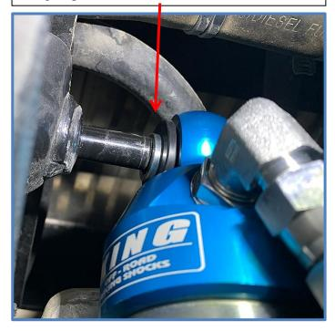
Factory nut will go on side with short bearing spacer.
