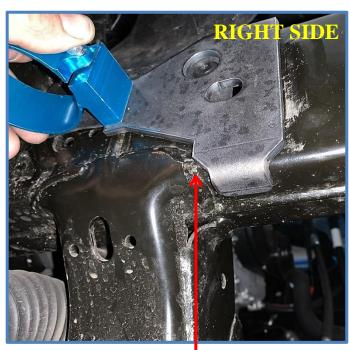
Make sure the bracket is sitting flat against the frame, remove any weld splatter and make sure bracket is not sitting on any welds.
