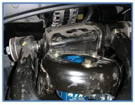
8. Reconnect upper A-arm to spindle, install nut and tighten to factory specs then insert cotter pin. Reinstall the ABS line brackets to the upper control arm and reinstall sway bar link to the spindle. Tighten all factory hardware to factory specs.
