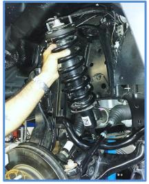
6. Install King Shocks. Be aware the shocks are side specific; make sure you are installing the shocks on the proper side. Start by placing the shock in position on the vehicle and install the factory lower mounting bolt.
