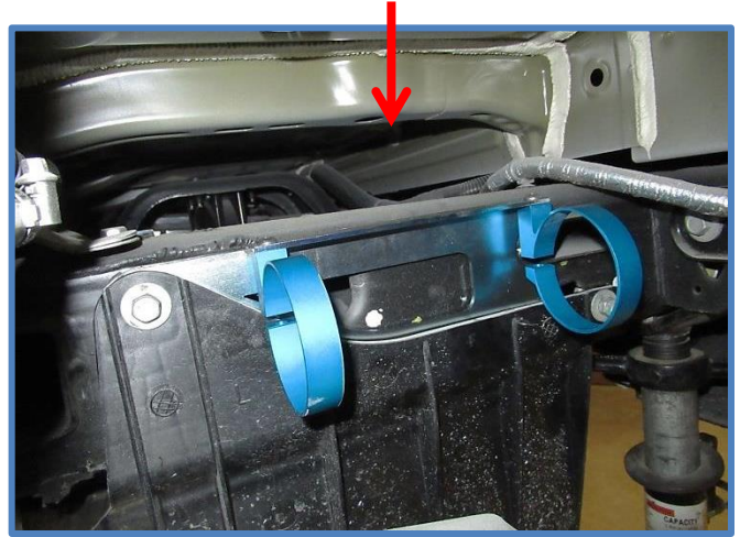
Left bracket installed with factory hardware.
