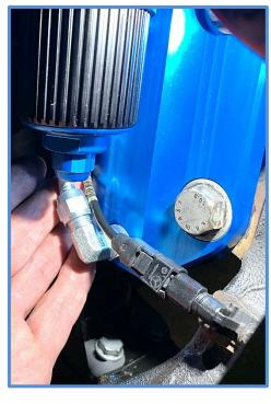
28. Attach ABS line to the shock – Slide ABS line holder onto tab on side of shock until it clips in.
