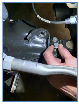
12. Place bracket on lower control arm as shown (brackets are side specific). Reinstall the factory bolt you just removed, place through the bracket and thread into lower control arm, leave loose for now.
