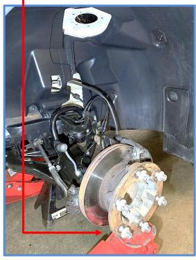
3. Remove the nuts from the lower mounting bolts using a 21mm wrench and socket. Remove the nuts but leave the bolts in place for now to hold shock.
