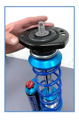
20. Place the upper washer on top of the upper mount with the flat side facing down.
