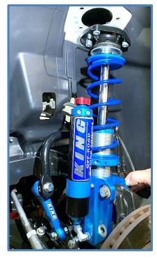
24. Make sure the steel inserts are in place and install the factory bolts through the lower mount. Thread nuts on but do not tighten yet.
