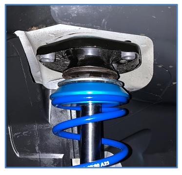
26. Reuse the factory upper mount plate inside the cab and the factory bolts to attach the upper mount. Install bolts and tighten to factory specs. When you are finished tightening upper mounts, replace tool tray, floor mats and trim pieces.
