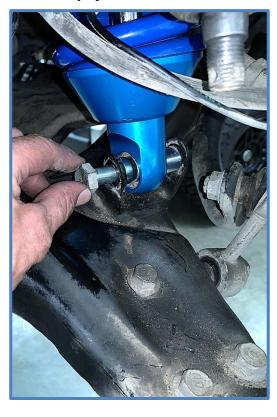
7. Reconnect upper control arm and tighten nut to factory specs. Install new cotter pin. Reroute brake/ABS lines and attach to knuckle. Secure brake lines to upper control arm with zip ties.
